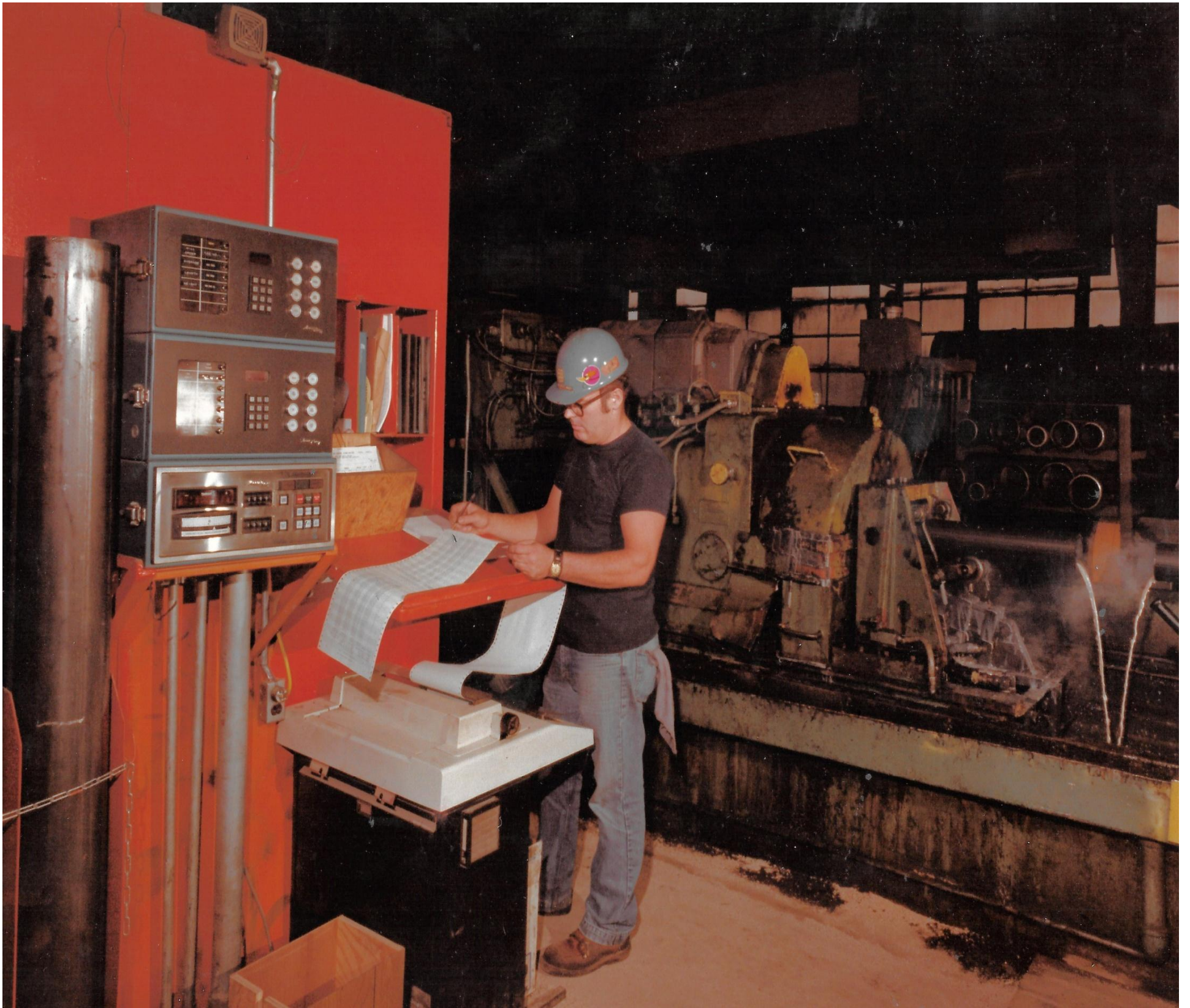
Operator's desk-TOP-530, Data CENTER 540-Auto-Control, Bottom-510 Gauge
